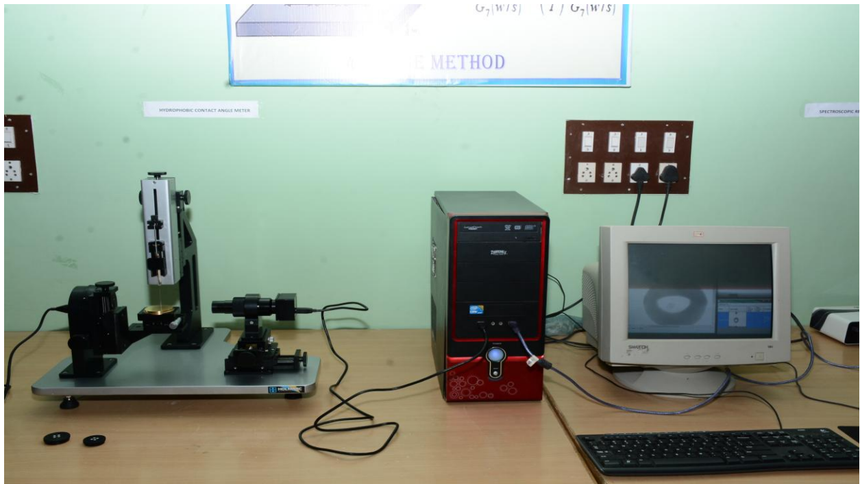
Contact Angle Meter
